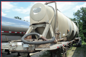
1977 Heil 1040 Cube, Steel Vessel, Spring Ride, Cement Service.
