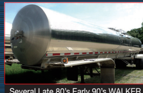
Several Late 80's Early 90's WALKER 6,000 gal, alum. frame & cradle, spring-ride, Dayton wheels.
