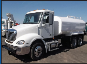
2009 FRTL Columbia 112, Mercedes OM460, 450 HP w/Jake, 10 spd, Air Ride Susp, 172" with, 107" cab to axle wheel base, 295/75/22.5 allum tires, 611114 ODO miles, A/C, Stk# V12F0574.....$65,000.
