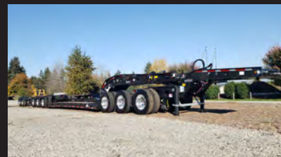
2019 Aspen 75T Lowboy Pkg (3+3+2) 24' x 8'6" Cantilever Deck, Dual Source Hyd, Hyd. Flip Neck, 3rd Axle Lift, A/R Susp, Disc Brakes, Jeep, and Tandem Axle Hyd. Relieving Booster.....P.O.R
