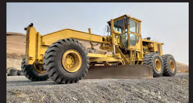
1973 Caterpillar 16G Motor Grader, CAT 3406 Engine, 250 hp, 23.5-25 Tires, 16' Moldboard, Pushblock, Accumulators, Hi-Pro Cab, Stk# PK3056.....$59,500
