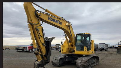
2015 Komatsu PC228USLC-10, 3022 hrs, 36" Dig Bkt, Combo Hydraulics, Wedgelock Hyd Coupler, 9'7" Stick, Hydraulic Thumb, Stk# PK1950 ..... $159,500
