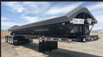
2019 RENN 3 & 4-Axle Side Dumps, 38' Tub, 1/4" Hardox, 90,000 lb GVWR, 33cuYds, Electric Tarp, Lift Axles, Ridewell A/R Susp, Aluminum Wheels ..... POR
