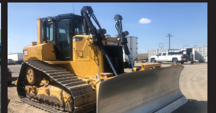
2014 Caterpillar D6T XW, 2993 hrs, VPAT Blade, Multi-Shank Ripper, 28" Pads w/ Carrier Roller, ARO Ready, Light Package, Stk# PK3155 ..... P.O.R
