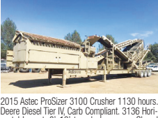
2015 Astec ProSizer 3100 Crusher 1130 hours. Deere Diesel Tier IV Carb Compliant. 3136 Horizontal Impact, 6'x12' two deck screen, Closed circuit w/magnet. Hydraulic tipping grizzly feeder. Hydraulic folding discharge conveyors. Remote Control. 200 Tons Per Hour. Like New.....$225,000.
