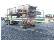
2014 KPI-JCI 6X20 Portable 2 DECK screen. Hyd legs. 60" under conveyor, 2 cross conveyors. Tandem axle chassis. $47,500.
