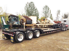
New 2018 Witcoz RG50 tri/A 50 ton Self contained Hyd removable gooseneck. 23' length X 8'6" width deck out riggers. 255/70/22.5 tires. FET paid.....$39,500.
