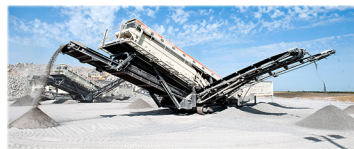
METSO ST3.8 Tracked Mobile Screen
