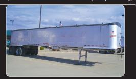
2005-2007 VANTAGE Frameless End Dump Trailers, 45 to 70 cubic yard capacity, empty weight 10,900, aluminum, tandem axles w/Hendrickson air ride suspension, 22.5 LP tires on all aluminum wheels, some w/Airgo tire inflation system, some w/combination tilt & swing tail gates, most w/liners.
