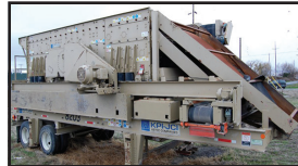
Used Portable Screening Plant , w/JCI 8' x 20' 3 deck screen 40 hp elec motor, 60" under screen conv 15 hp electric motor, cross conv, discharge chutes, walkways mounted on tandem axle trailer. P.O.R.
