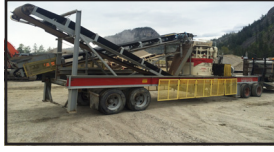
Used Portable Cone Plant , w/45" El-jay Cone Crusher, 125 hp, under cone conveyor and incoming feed conveyor, mtd on tandem axle, ..... P.O.R.
