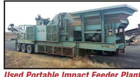
Used Portable Impact Feeder Plant , w/Inertia 50" x 66" Horizontal Impactor diesel power, 50" x 18' VGF, 48" discharge conveyor, mounted on triple axle trailer..... P.O.R.
