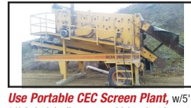
Used Portable CEC Screen Plant , w/5' x 14' 3 deck incline screen 20 hp electric motor 30" under screen conveyor discharge chutes walkways mounted on single axle trifer. P.O.R.
