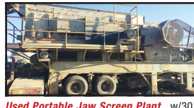
Used Portable Jaw Screen Plant , w/30" x 42" Pioneer Jaw Crusher 150 hp, 6' x 16' Eljay 2 deck Heavy scalper 40 hp, 42" discharge conveyors 15 hp, leveling cylinders, mounted on tandem axle trailer... P.O.R.
