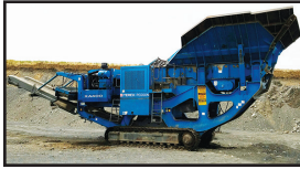
Used Portable Track Mtd Jaw Feeder Plant , Pegson XA 400 28" X 44" Jaw crusher vibratory feeder powered by Cat motor..... P.O.R.
