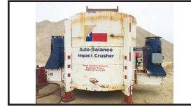
Used Portable Impact Plant , w/Texas Crusher VSI two 200 hp electric motors, 42" discharge conveyor 15 HP electric motor, mounted on tandem axle trailer..... P.O.R.
