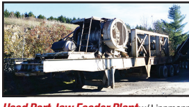
Used Port Jaw Feeder Plant w/ Lippmann 30"x62" Jaw Crusher 200 hp, 50"x20" VGF 40 hp, hopper, 48" discharge Triple axle... P.O.R.
