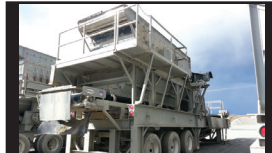
Used Cone Screen Plant , w/Symons 41/4SH Cone, 200 hp, Eljay 6'x16' 3 deck screen 40 hp, 48" discharge conv, triple axle trf... P.O.R.
