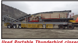
Used Portable Thunderbird closed circuit plant , w/1200 LS Cone Crusher, 5X16 3-deck screen, under crusher conv, CC conv, under screen conv, leveling cylinders, mtd on triple axle trf..... P.O.R.
