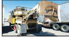
Used Portable Impactor plant , ISC 77 VSI 300 hp electric motor, 42" discharge conveyor 15 hp electric motor, mounted on tandem axle trailer ..... P.O.R.
