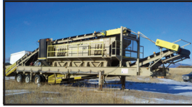
Used Portable Screen Plant , 6'x20' JCI, heavy scalper, 50 hp., 60" discharge conv, (2) ea. 42" cross conv, 42" feed conv, triple axle trailer, ..... P.O.R.
