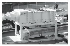
Twin hydraulic units with two 125hp electric motors power each shaft independently, shafts each have 13 3" - cutters, gear reducers generate over 200,000 lbs/ ft of torque/shaft, two 28' conveyors remove and load shredded material. Extra blade sets and generators available separately. 2007, 975 hrs, ............\$385,000.
