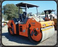
2009 Hamm HD120VO Articulated Vibratory Tandem Roller w/134 HP Deutz TCD2012 Diesel, Hydrostatic Drive, Rated 3200 vpm/41,850# Max Centrifugal Force, 31,500# Tare Weight, 78" Drums w/ Dual Drum Drive, Water System, ROPS, Lights..........................\$60,000.
