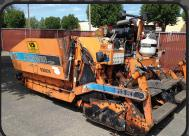
2001 Gilcrest 813RT ProPaver Crawler Asphalt Paver w/ 80HP Turbo Diesel, Hydrostatic Drive, 12" Flat Pads w/ Bolt-on Urethane Street Pads and Track Covers. 7.5 Ton Hopper 8 to 14-ft propane heated hyd screed. Extensions to 16-ft. Dual Auto Conveyors, truck hitch, work lights. 1458 hours. ......\$20.000.
