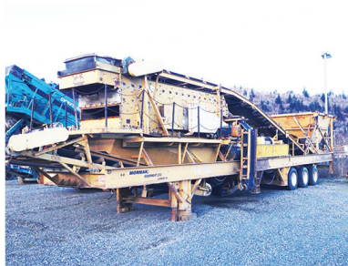
1995 Cedarapids 5 x 16 triple deck closed circuit crushing plant. 45" Roller one II changed in 2004, major overhaul done in winter of 2013. Excellent Shape
