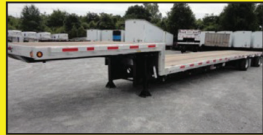
2016 DOONAN Platinum , 50.5' x 102", Tandem Sliding Spread Axle, 17.5 Tires, Al. Outside Wheels, Apitong Floor, 10' Upper Deck, 40.5' Lower Deck, Stk #16046
