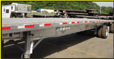
2016 CHAPARRAL II , 48', Air Ride Susp, 295/75R22.5 Tires, New all aluminum, Front Left Axle, Fixed Spread. Stk #1697-09337
