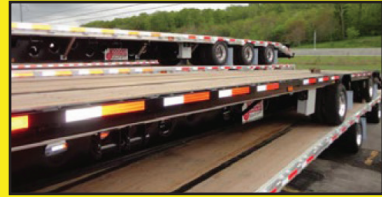
2016 DOONAN Black Gold , 50'6", Hendrickson Suspension, Spread Fixed Axle, Apitong Floor, New All Steel Beavertail, 17.5 Tires, Top Deck Ramps, Container Locks. Stk #1622-09104
