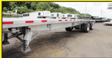
2016 CHAPARRAL II , All Aluminum 53ft Flatbed, Air Ride Susp., All Aluminum Wheels, 295/75R22.5 Tires, Fixed Spread. Stk #1695-09312 ... $39,235.36
