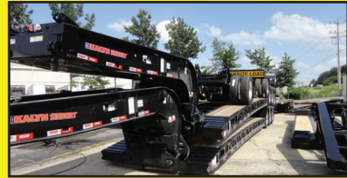
55 Ton Kalyn/Siebert , 3 axle, Adjustable 5 position ride height. Swing clearance 108". 6" ground clearance. 14 pair d-rings. Alum outside wheels, 26ft main deck. 1-3/4" Apitong floor. 8 ft I-beams on 24" centers. Honda power Pack. 5 year pro-rated Frame warranty Stk#1725-08290
