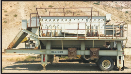
Portable El Jay 5' wide x 16' long Three Deck Horizontal Screening Plant, under screen discharge conveyor, product chutes, walkways, single axle. (UT).....$35,000
