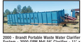
2000 - Brandt Portable Waste Water Clarifier System - 3000 GPM Mdl 56" Clarifier - 11' x 56", 15 h.p. electric / hydraulic, 11" mud hopper, electronic controls, flocc mixing & injection system, 3 axle chassis, bolt on support structure, walkways & stairs, (Oregon) $125,000
