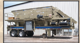
JCI 6203-32 Screen Plant w/Switchgear, Portable
