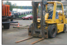
CAT 80E Forklift, open ROPS, 8,000-lb. cap., 4-cyl., propane ..... .....$5,900.
