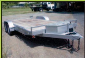
2008 MORGAN BUILT Tilt Trailer, sn 105-5662, 9,980 GVW, 19'2" tilt deck, elec. brakes, toolbox, 225/175x15....$6,500.
