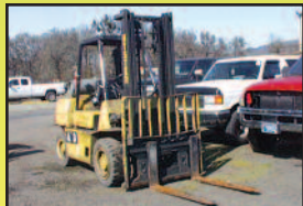
HYSTER 8,000-Lb. Forklift, LPG, 12' lift, 2-stage mast, sideshift, sn G005D-05830S.....$9,500.
