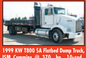
1999 KW T800 SA Flatbed Dump Truck, ISM Cummins @ 370 hp., 10-spd., 12,000-lb. front, 23,000-lb. rear, 18' steel flatbed w/hoist, removable sides, toolboxes, dean truck, 35,000-lb. GVW .....$18,500.
