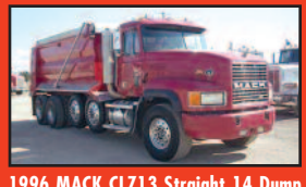
1996 MACK CL713 Straight 14 Dump Truck, E7 400, Jake, 12-spd., 20K-lb. frt., 46K-lb. rears, Hend. susp., Reliance 17' dump box, (2) 12K-lb. steerable lift axles, 82K-lb. GVW.....$29,500.
