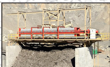
New Filter Press, an excellent alternative to a belt press, dehydrates all types of slurry and reduces water costs by up to 90% by recycling it.. Rent or Buy - P.O.R.
