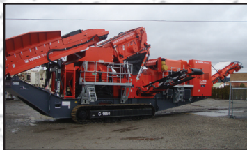
New FINLAY C-1550 Track Mounted Cone Plant, w/Terex 1300 remote adjust cone crusher, Cat C-15 dsl, low level lg. hopper with belt feeder & metal detector, & 8' x5' pre-screen unit folds for transport..... Rent or Buy - P.O.R.
