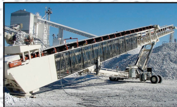
2012 Superior 36"x150' Telescraper with PLC PilePro controls, FD axle, power raise/lower, power travel, 4WD... P.O.R.
