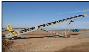
30" Wide x 60' Long Radial Stacker, 15 HP Motor, Adjustable Height Undercarriage..... For Rent or Sale
