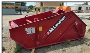
McLanahan VD18 6' Wide x 12' Long Dewatering Screen with Twin 8 HP Electric Motors, Urethane Media
