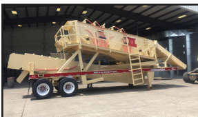
Portable Wash Plant with 5' Wide x 16' Long Triple Deck Wet Screen, 36" x 25' Sandscrew..... For Rent or Sale
