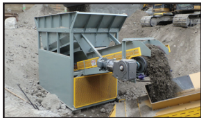
Feed Hopper with 36" Wide Variable Speed Belt Feeder, Optional Grizzly Available..... For Rent or Sale
