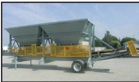
Portable 2 Bin Blending Hopper with 30" Belt Feeders, 36" Collecting Conveyor..... For Rent or Sale
