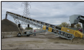
36" Wide x 80' Long Portable Radial Stacker, Self-Contained with 49 HP Diesel Engine..... For Rent or Sale
