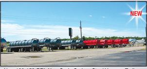
New 130-150-BBL Non-Code Carbon Steel Vacuum Trailers - IN STOCK or BUILT TO YOUR SPECS!
