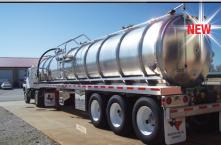
NEW ITT 8000 Tri-Axle Aluminum Vacuum Trailers. 11R24.5 steel disc, air-ride - BUILT TO YOUR SPECS!
