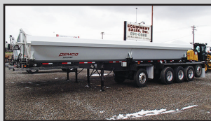
2020 DEMCO SS445, 44' Quint Axle, (5) Axles, Air Lift 1st & 5th Axle, AR Susp, 37" Tub, 6" Cylinders, Elec Tarp Sys, Tarp Lockout Sys, Elec Over Hydr Valve, Possible 105K GROSS w/ 4 Axle Tractor, GVWR 112K lbs...$78,500 + F.E.T.
