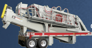
Portable 516Wash Plant 5'x16' - 3-deck screen, 36"x25" sand screw, and optional hydraulic slurry box.
