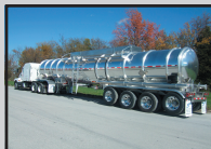
11,000-GAL. 2 COMPARTMENT ALUMINIUM DOT-407
