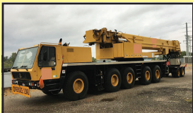
1996 GROVE GMK5175 All Terrain Hydraulic Crane - Cummins, 161' boom, lattice jib, 75 ton block, dual cable winches, 99K# weights.....$340,000.
