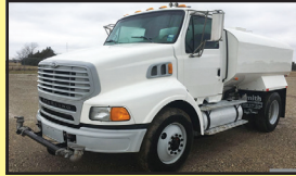
2001 STERLING A9500 S/A WATER TRUCK - Cat C12, 355 hp, eng brake, 7 spd, A/R, PTO pump, FS&R sprays, 12K FA, 20K RA, 2500-gal tank, 371K miles.....$34,500.
