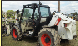
2006 BOBCAT V518 4x4 Reachlift - Perkins 1104C-44T, 100 hp, 5500# cap at 17', cab with AC/heat, choice of bale grapple or pallet forks, 3732 hours...$29,500.
