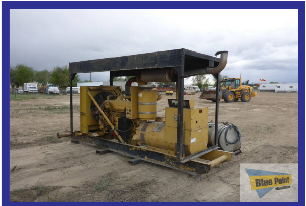
Kato 247 KW Genset Generator 250-749 Kw/310-950 Kva. Powered by an 8 cylinder Cummins NTC855C diesel Utah .....$7,500
