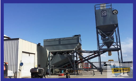
Ross Bandit Portable Concrete Batch Plant manual controls, 60 ton silo, single load portability, digital water meter and scale, overhead agg. storage. ..$125,000
