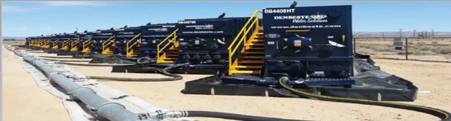
1200c.f. (300 brrl) Portable silo, 8'-6" wide x 13'-6" tall and 35'-0 long. Single hopper with three hoppers-7" carry over auger under hoppers, 5hp 480v motor and gearbox, 10" discharge hopper with 10hp 480v motor with gearbox, chain drive, DSS lube block seals, manuals slide gates on each hopper, (36) air fluidizers with manifold on the cones, 150sq. ft. dust collector with electric vibrator and cleanout compartment, NEMA 3r electric panel with disconnect and silo controls. ...$43,000
